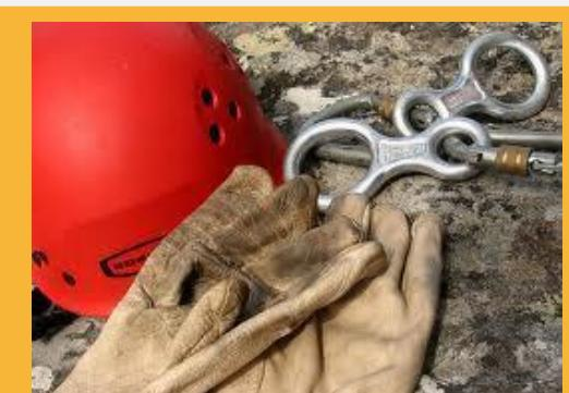
*Helmets, Figure of eight descending devices and leather gloves used for abseiling.*
